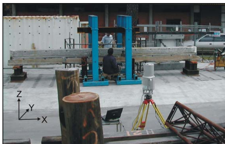
Figure 2: Concrete beam and the Riegl LMS-Z210
