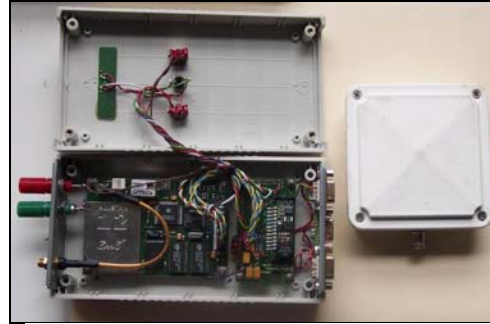
Figure 3: Prototype Locata (receiver) hardware.
