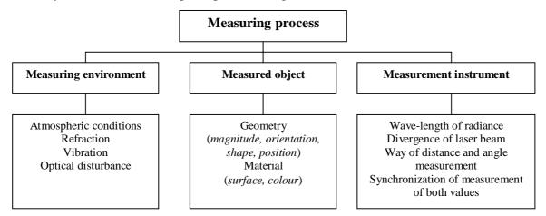
Fig. 2: Element properties of measurement process
