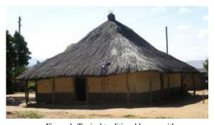
Figure 1: Typical traditional house, with raw bricks walls and thatch roof.
