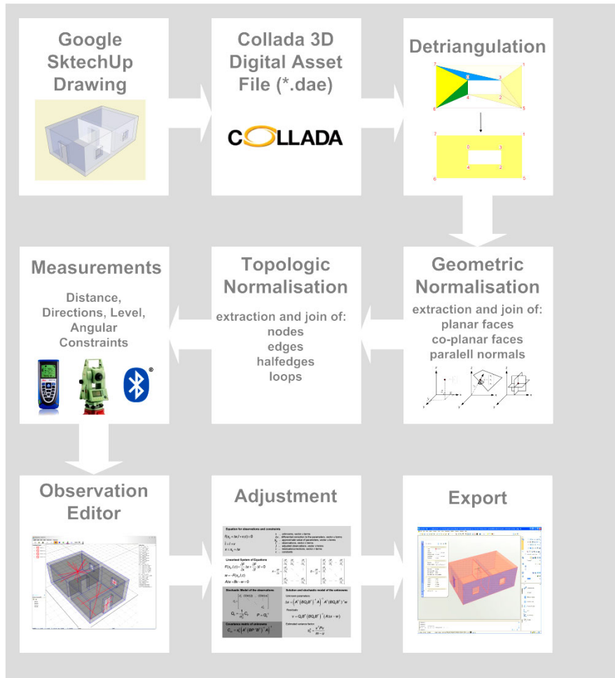
Fig. 5: Exemplary workflow to test the data model
