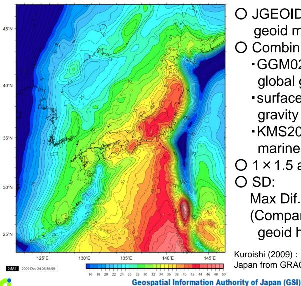
O JGEOID2008 is the latest gravity geoid model by GSI for Japan.
