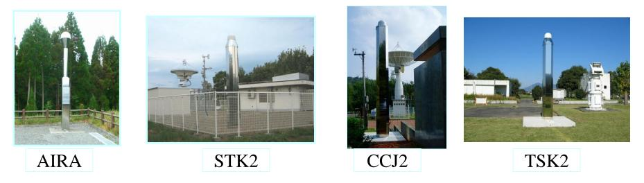
Receiver : Trimble NetR9 Antenna : Trimble Choke Ring (TRM59800.00) Differences from GEONET stations : precise external frequency and radome
