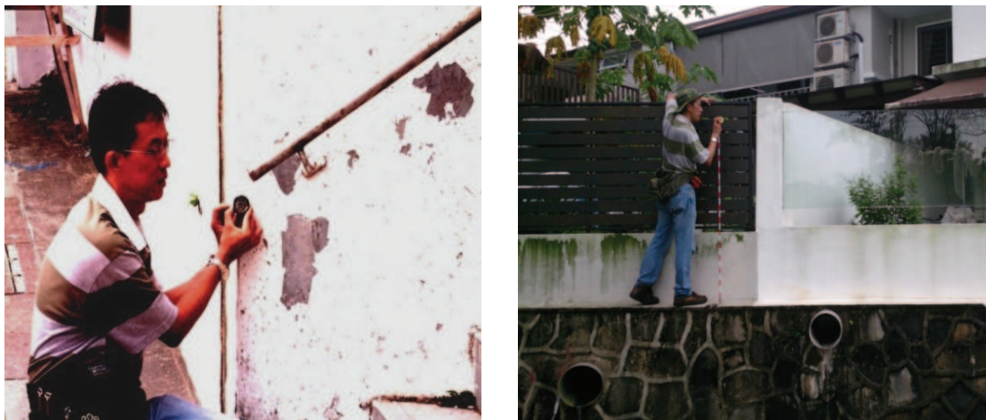
Figure 2: Surveyors using Total Station to pick up location of encroached structure by placing a mini prism on the encroached object.
