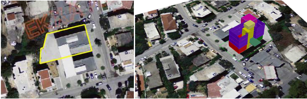
Figure 4. Adjustment of real property 3D model in HGRS87: Left: Location of real property coordinates in GGRS87 in the VLSO of the HC. Right: Real property 3D model after the coordinate adjustment placed over HC VLSO
