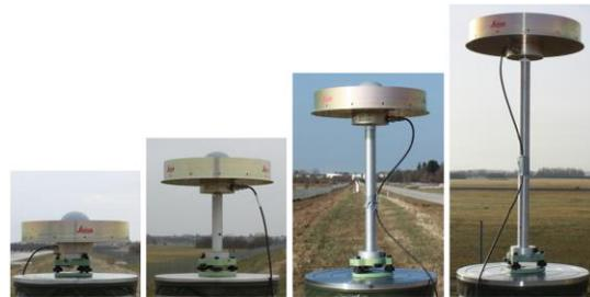
Fig. 1 Set-ups for Leica AT504GG Choke Ring antenna.
