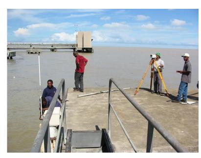
Tide Gauges sited away from river mouths – areas of strong wave action or currents Considerations: Subsidence and disturbance to wharf Slipping of tide gauge zero mark over time – damage Important to have nearby BM on bed-rock away from wharf
