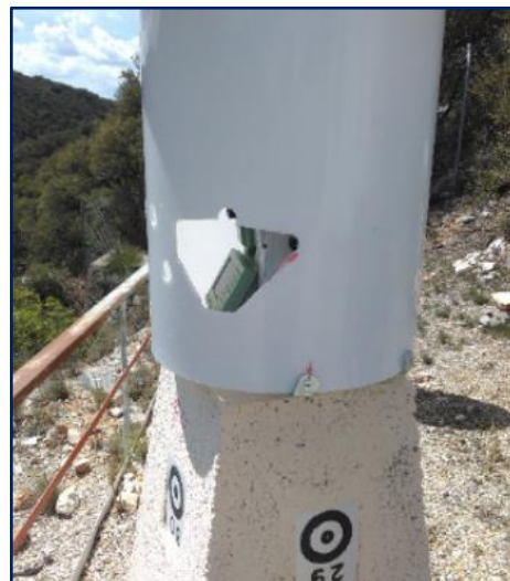
Figure 5. Total station located on survey column P04
