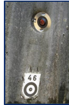
Figure 4. Lava rosette and associated prism reflector
