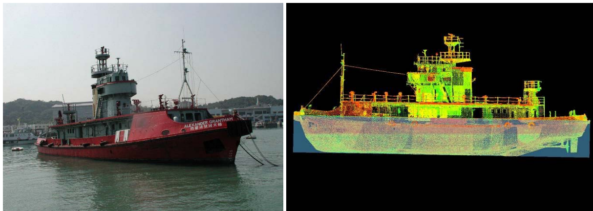
Fig 17. Fireboat “Alexander Grantham” (left photo) and its Point Clouds (right photo)
