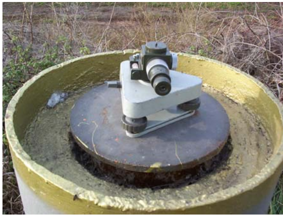
Figure 2-2: The view of the top of the pillar with fixed geodetic tripod
