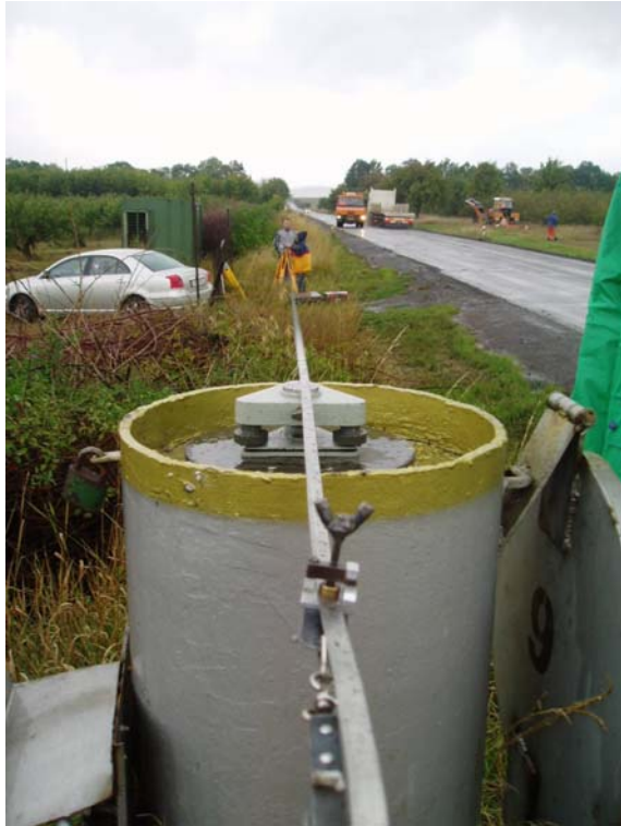
Figure 3-1: Measuring of the distance from the pillar no. 6 by invar tape
