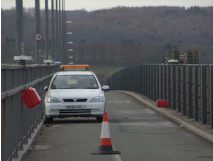
Figure 3. Light-Weight Leica Choke Ring Antennas on Bridge Railings.
