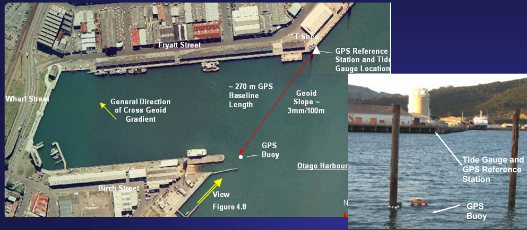
Water Level Measurement and Tidal Datum Transfer Using High Rate GPS Buoys
