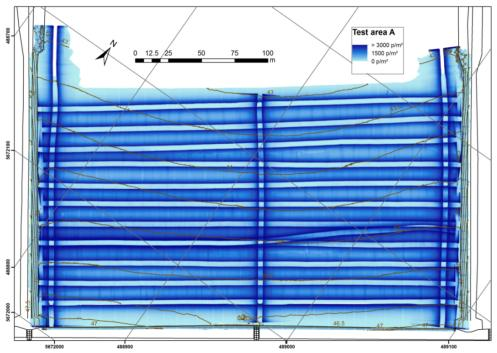
Figure 4: Point density map of the MTLS data (per m<sup>2</sup>)
