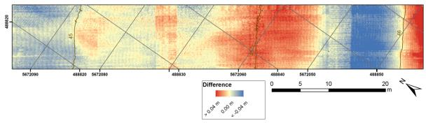
*Figure 6: Differences in altimetry between MTLS data and STLS data for the small area on the beach*
