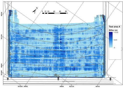
Figure 5: Standard deviation map of the MTLS data (per dm<sup>2</sup>)
