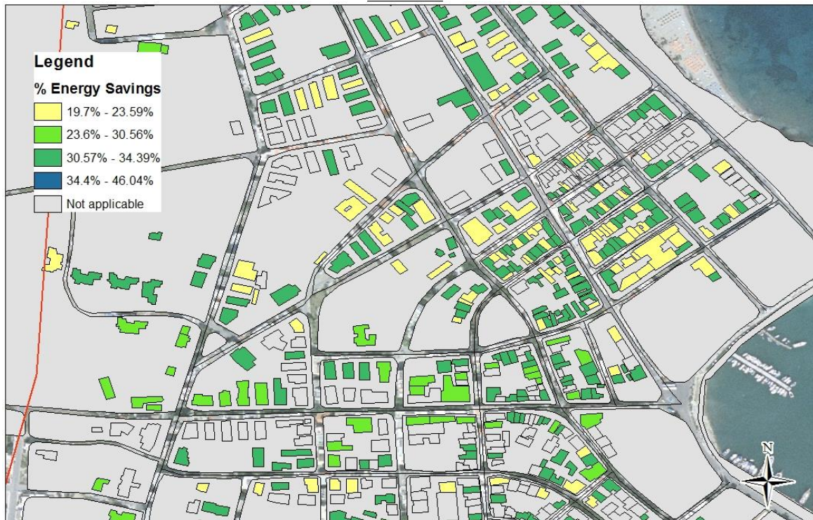
Figure 6 - Energy savings per residence after installing solar thermal collectors for DHW
