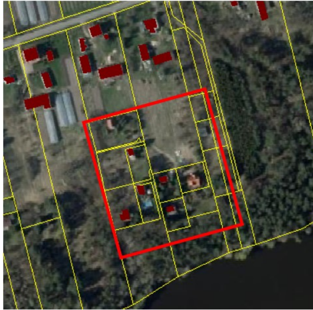
Fig. 4. Example of building plots without access to the public road in the Kikoły village, Pomiechówek commune
