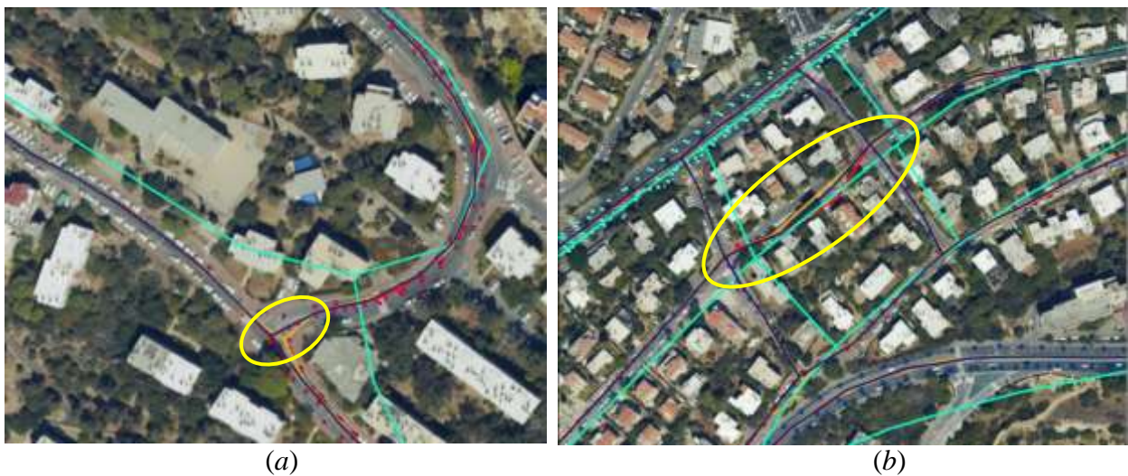
FIGURE 7. Example of the realignment results (a) the impact of iterations (b) the impact of sparse GPS points.
