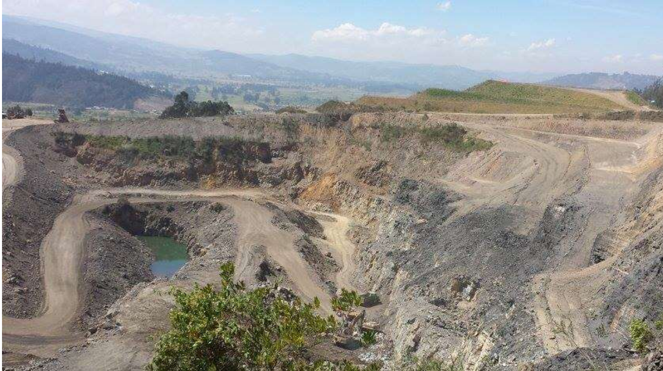
Design of terraces of constant height and berms in a single nibe
