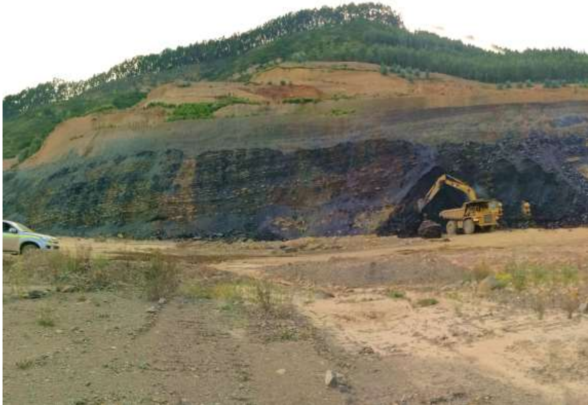
Geometric cut with heights and widths of berms established in the design.
