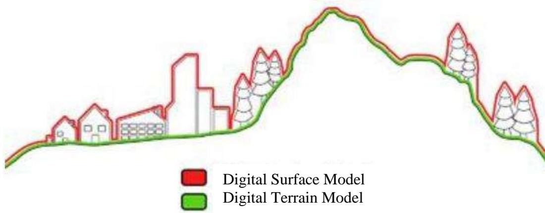
Using the Digital Terrain Model and Digital Surface Model, calculations are made for the difference between the two. This provides a representative feature height that is used in capture interpretation. When the height tool is activated the cursor provides the height in metres (m) as the cursor is moved over features, the number adjusts dynamically to display the correct figure.
