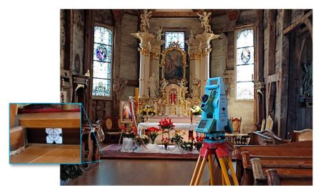
Fig.5. Leica TCRP 1201+ total station in the station in the center of the nave; on the left side, a reflective foil target – one of the points of reference.
