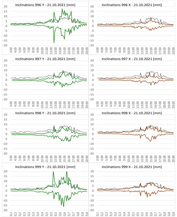
Fig. 8. Indications of the maximum inclinations of the tested object in 4 places (sensors 996, 997, 998 and 999) at the ceiling level, corresponding to the readings from the weather station in Fig. 7; thin black line indicates gusts of wind from weather station.
