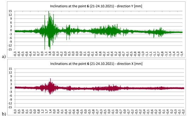
Fig. 6. Selected diagram of structure vibration at point 996 in the 3-day recording period during strong winds: a) inclinations across the church, y axis direction, b) inclinations along the church, x direction. Angular values converted to horizontal displacements at a height of 7 m.
