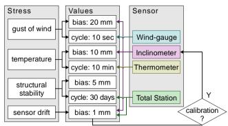
Fig. 4. Block diagram of the measurements: "bias" means the permissible values of displacement at the ceiling level, "cycle" defines the interval of data acquisition.
