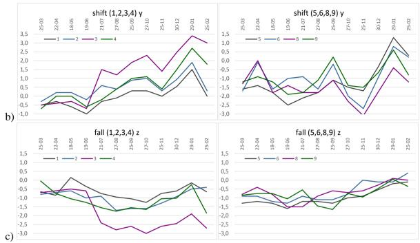
Fig. 7. Graphs of long-term displacements of points measured using the tachymetric method: a) movement in the x-axis direction, b) in the y-axis direction, c) settlement – points from the P section on the left, points from the N section on the right; each measurement with an average error of  $\pm 1$  mm.
