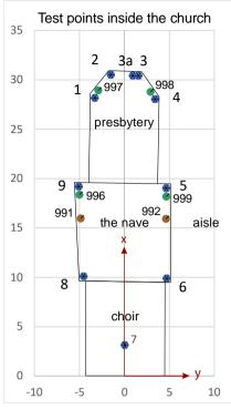
Fig. 3. Distribution of test points - sights and inclinometers - on the object (explanations in the text)
