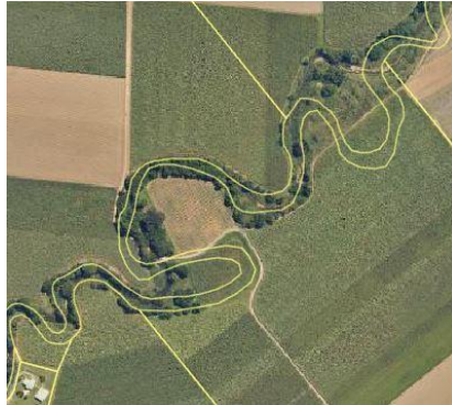
Figure 2(a): Separation of riparian boundary to the natural feature, Edmonton Qld (Source: Queensland Globe)
