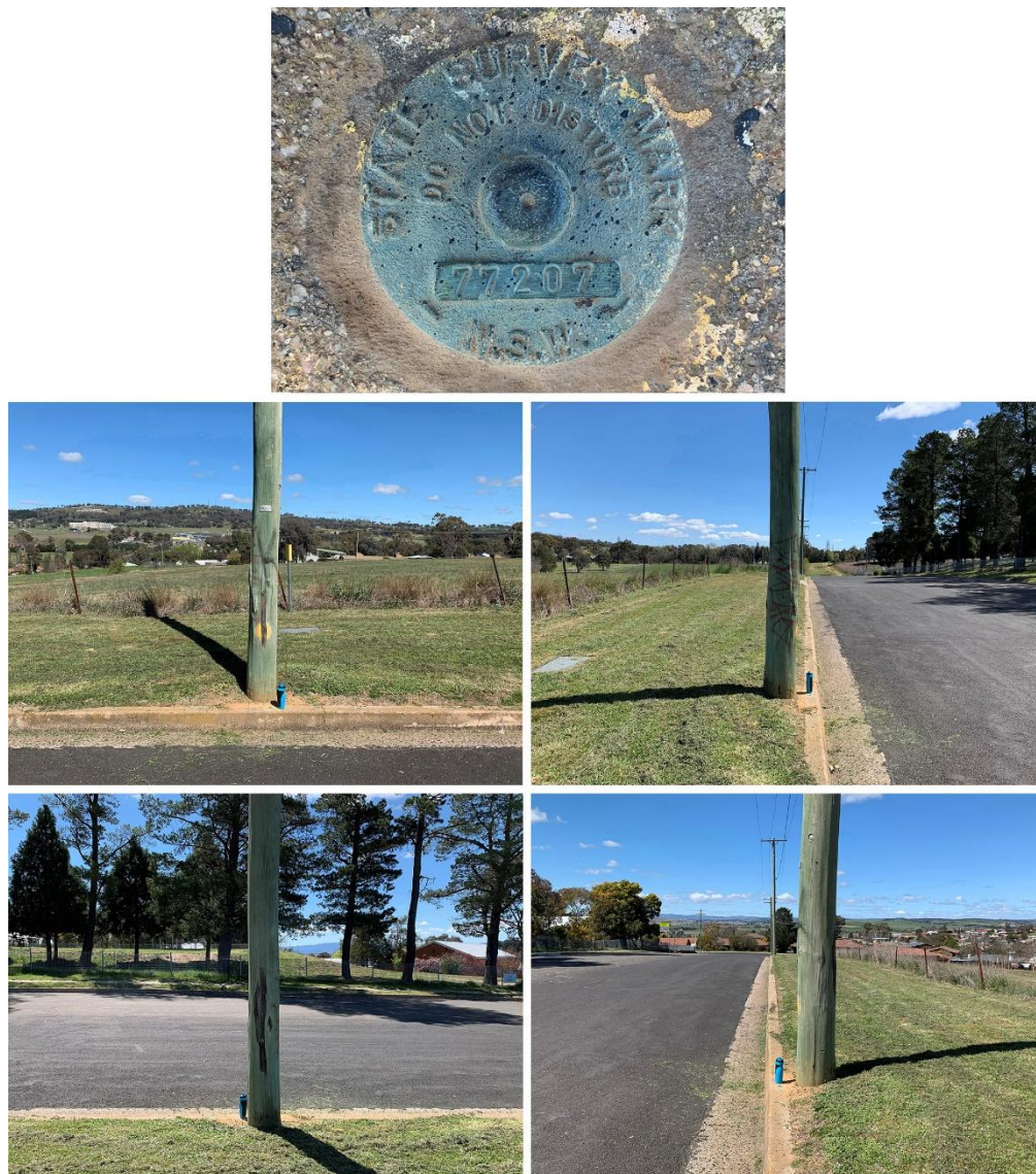
Figure 4: Photos taken at SS77027, showing a close-up of the SSM plaque and views from four perpendicular directions, using the kerb for orientation and a colourful water bottle indicating the mark location.
