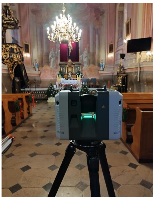
Fig. 1 Lector RTC 360 Scanner at the abbey to Capture Point Clouds
