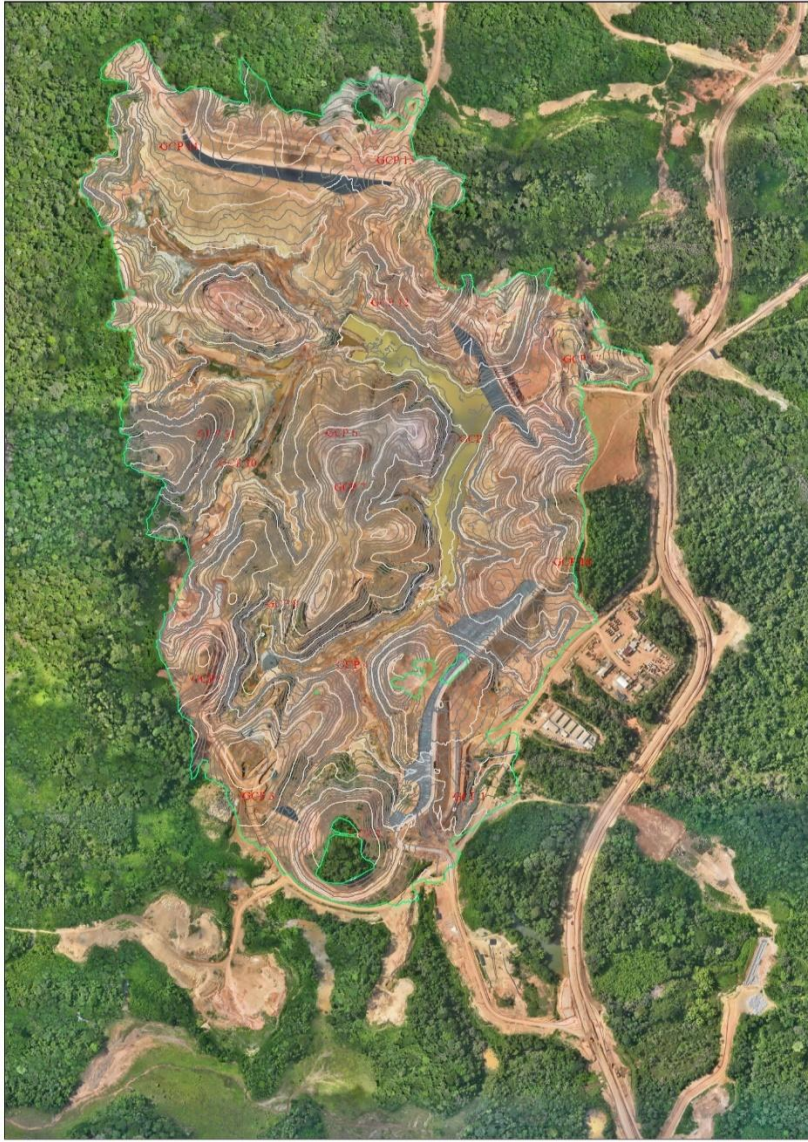
Contours from GNSS survey overlay on tiff.
