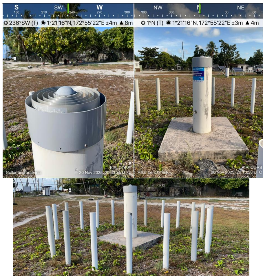
Figure 2: KIRI CORS choke-ring antenna (top left), monument pillar (top right) and protective pillars around CORS (bottom)
