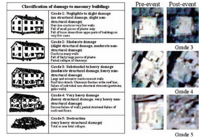
Figure 4.2.12: Classification of damaged buildings (EMS1998) and pre and post visual interpretation (Yamazaki et al., 2005)
