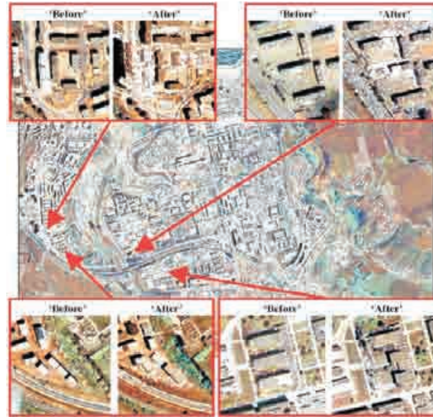
Figure 4.2.11: Example of earthquake damage assessment in Boumerdes, Algeria (Adams, 2004)
