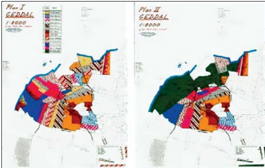
Figure 7.6 Land consolidation converts an area of scattered land parcels, left, into more homogeneous holdings, right, to optimize farming.
