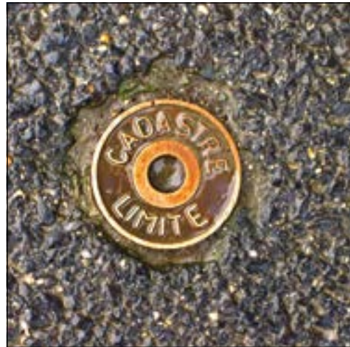
Figure 12.13 An on-the-ground boundary mark with a metal pin is used in Switzerland.
