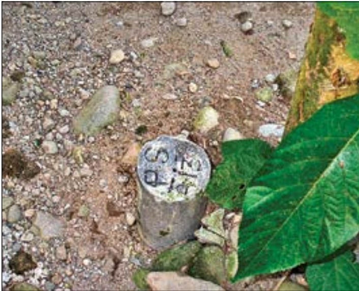
Figure 12.14 A concrete boundary mark that numerically identifies the mark is used in the Philippines.
